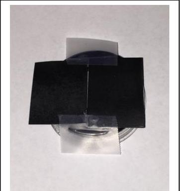
Figure 8a: Slit formed by 2 card rectangles
