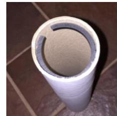
Figure 6a: Put a C-Ring into the tube.
