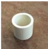
Figure 3: 1 inch section of 1 inch diameter PVC pipe
