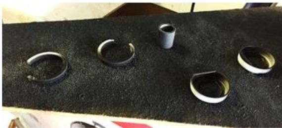
Figure 5: Paint all the plastic parts flat black
