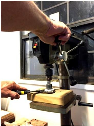
Figure 7: Drilling a 1" hole in the plastic endcaps.
