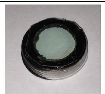
Figure 10: Hot Melt Glue the CD to the other end cap (inside).
