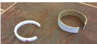
Step 2: Make 2 C-Rings to hold the lens in. You have two options: make them from the cardboard mailing tube or from the 2" PVC tube. The cardboard retaining rings are easier to make, but often the cardboard delaminates. Also, they must be glued in as they do not hold well against the side of the tube. The PVC tubes are much harder to make, but don't need to be glued in and hold the lens better. I have the equipment to make the PVC ones so that is what I use.
