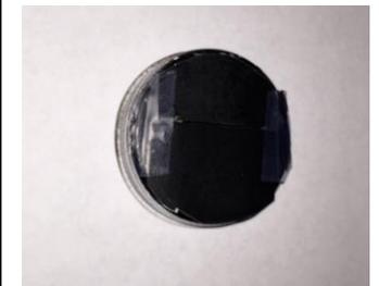
Figure 8b: Trim the tape and rectangles flush.
